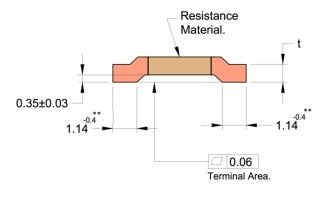
\*\* Tolerance for t≤0.67 mm, for t>0.67 mm applicable tolerance is +0/-0.7
