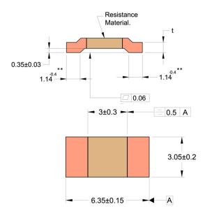
Dimensions are in mm, See table 2 for thickness.
